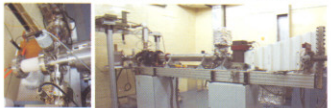
Fig. A.8.3: Electron gun developed by PHPMS (shown on left) integrated with 10MeV LINAC at RRCAT.
