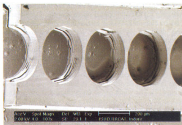
Figure T.1.15: Compound refractive lens fabricated in PMMA.
