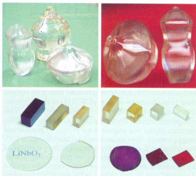
Fig.T.2.4 : The as grown crystal boules and elements of undoped and doped \text{LiNbO}_3
