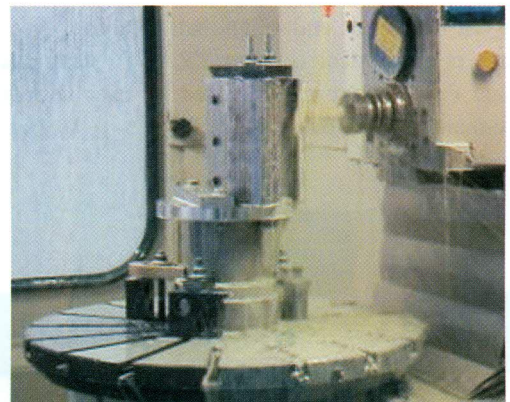
Fig A.14.4: Machining of Quadrupole Magnet pole blocks on 4 axes CNC machine
