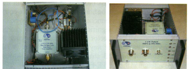
Fig. A.8.4: 1 kW amplifier system assembled inside the half 19 inch 3U chassis.
