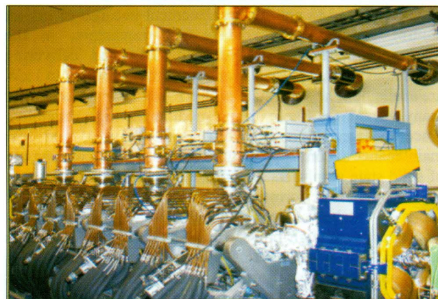
Fig. T.1.1: High power Klystron and cavity based RF system in Indus-2 SRS
