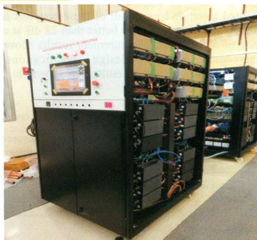
Fig. T.1.3: 13 kW solid-state RF amplifier developed unit
