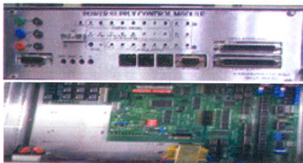
Fig.A.12.1 External and internal view of Power Supply Control Module (PSCM)
