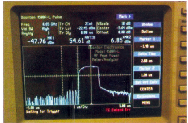
Fig. A.16.2 : Klystron RF output @ 30MW at 2856MHz, on a peak power meter.
