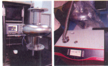
Fig.A.3.3: (a) The prototype cavity undergoing RF inspection and (b) Cavity under vacuum leak testing.
