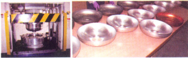
Fig. A.3.1: (a) Half-cell forming; and (b) Formed half cell in aluminium, copper and niobium.
