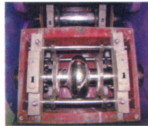
Fig.A.4.2 (a) : Cavity loaded on barrel polishing machine
