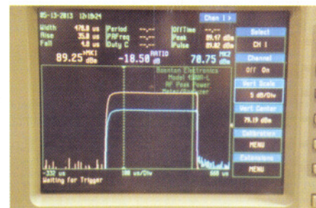
Fig. A.6.5 : Klystron RF output on a peak power meter, Yellow: forward power@ ~860kW, Blue: Reflected power @ ~12kW
