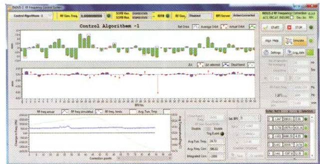
Fig.A.4.2: GUI snapshot of average orbit drift correction system in Indus-2.
