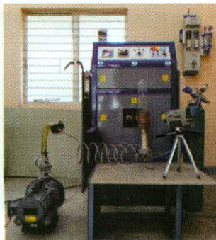
Fig. L.15.1: Partial pressure induction brazing system.
