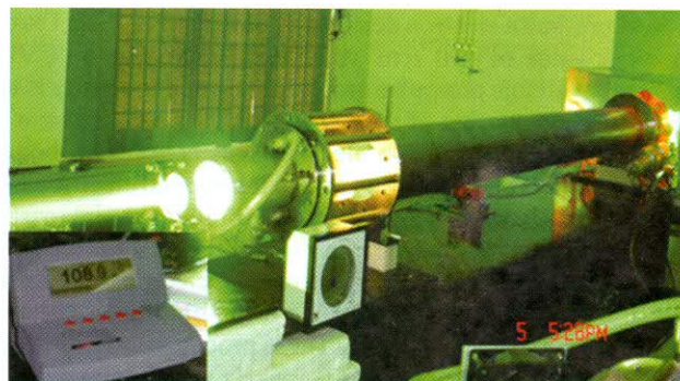
Fig.T.1.1: Photograph of 100 W average power class (max.: 110 W), 18 kHz PRR Copper-HBr laser developed in RRCAT
