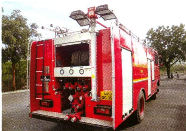
Picture I.3.2: Water pump and light mast
