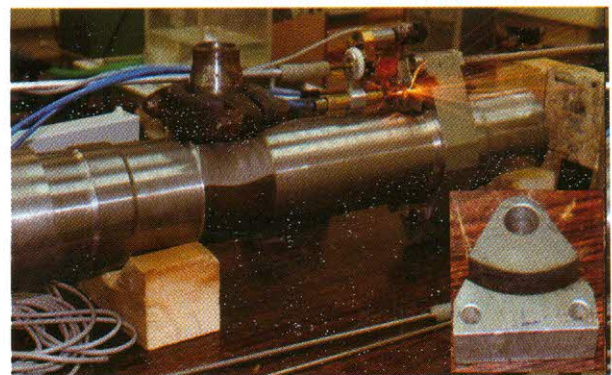
Fig. L.1.1: Laser cutting mock-up of triangular fixing block of coolant channel of pressurized heavy water reactors and the inset shows the laser cut triangular block
