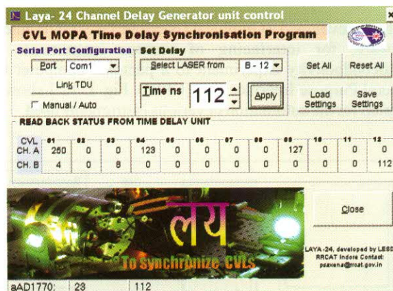
Fig. L.13.3: Master control GUI-LAYA -24 for TDUs
