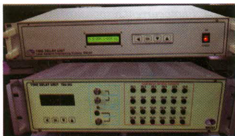
Fig. L.13.2: Time Delay Units of 2- and 24-channels
