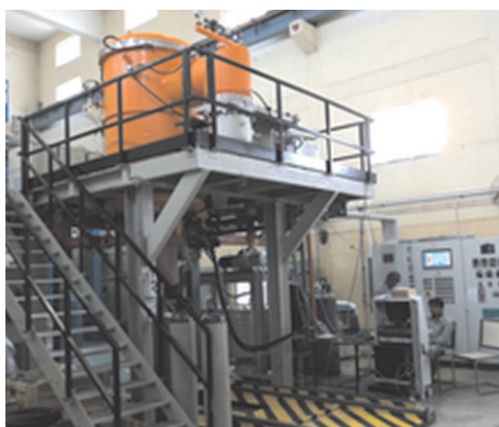
Fig. I.3.1: The furnace during the installation phase
