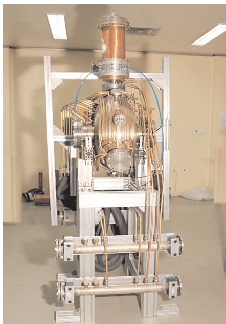
Fig. A.4.1: Fully fabricated RF cavity with Power coupler sensing couplers and cooling circuits.
