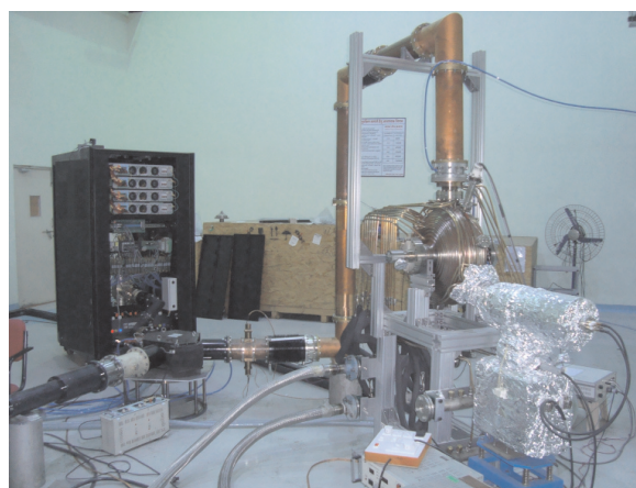
Fig. A.4.2: High power test set up for RF Cavity.
