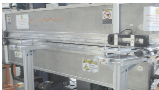
Fig. A.9.3: IR-FEL undulator with vacuum chamber
