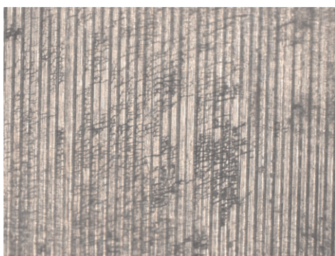
Fig. L.10.2: SCC on machined internal surface of SS tube.
